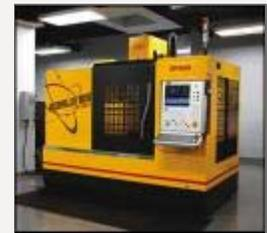
The CNC on this VMC uses constant-velocity technology to maintain high average machining speeds.
