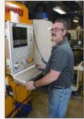
Mr. McCracken stands at the Revolution control. Unlike conventional systems, this CNC calculates look-ahead before program start and adjusts cutter movement as the machine runs.
