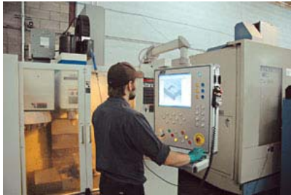
MTI's constant velocity controller (shown) retrofitted to a Fadal vertical machining center produced many benefits, including quicker cutting times. Gains vary widely, but some applications have been up to 70% faster. Source: Fidelity Machine
