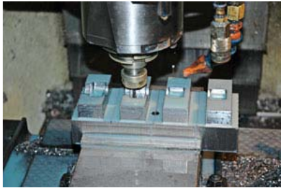
Mechanically, Fidelity's original machines were capable of moving at 300 to 400 inches per minute, but the outdated controllers weren't. MTI's constant velocity controller is built for speed and is appropriate for applications like this: machining strain relief inserts for cable overmolds. Source: Fidelity Machine
